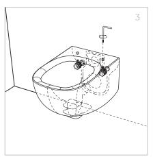
3. Tighten the pin inserting the key in the installation holes of seat cover
